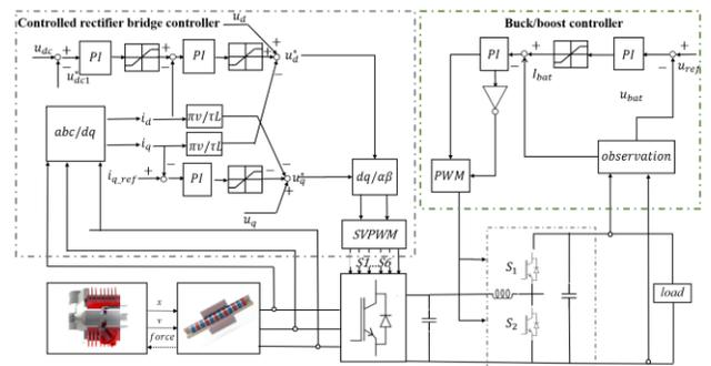
Fig. 4 Two-stage rectifier circuit topology
