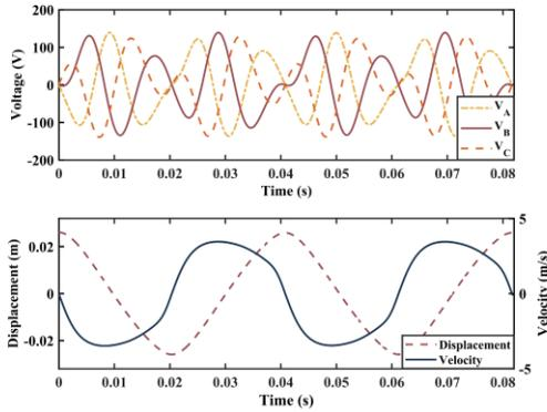
Fig. 7 No-load characteristics of linear generator
