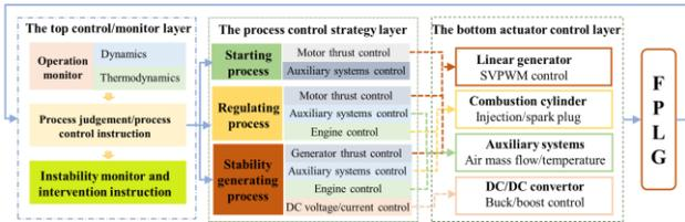
Fig. 2 Proposed FPLG control structure
