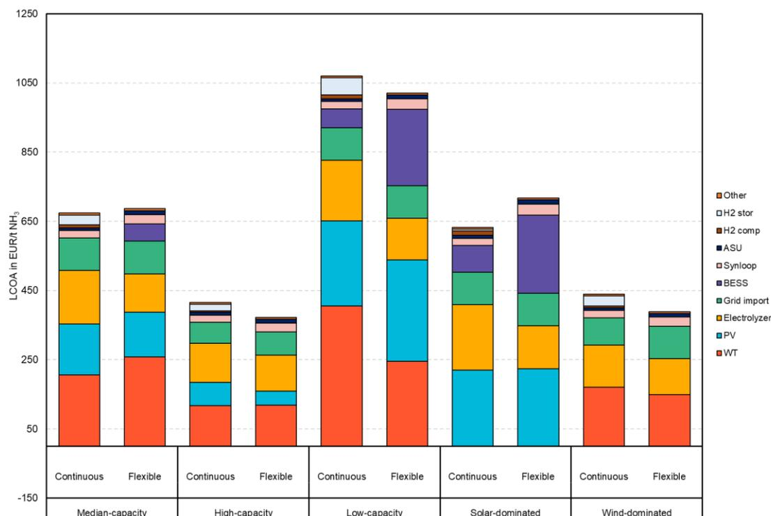
Fig. 3: LCOA for continuous and flexible electrolytic ammonia plants in different representative synthetic regions.
