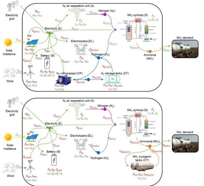
Fig. 1: Electrolytic ammonia plant subsystems. (a) continuous plant; (b) flexible plant. Variables in red indicate the decision variables of the model, while variables in green are input parameters for the optimization model.
