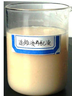
Fig. 4 Clean fracturing fluid with a glue breaker configuration. Samples were formulated into a bio-clean fracturing fluid at concentrations of 3.0% and 4.5%. Both formulations exhibited a pH of 7, with apparent viscosities of 43.5 mPa·s and 57.0 mPa·s, respectively.
