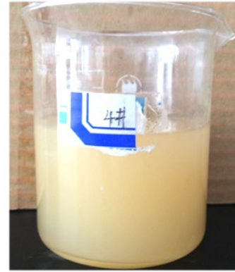
Fig. 3 Appearance of fracturing fluid post-gel breaking.
