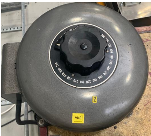
Fig. 2. Variable Voltage Transformer
