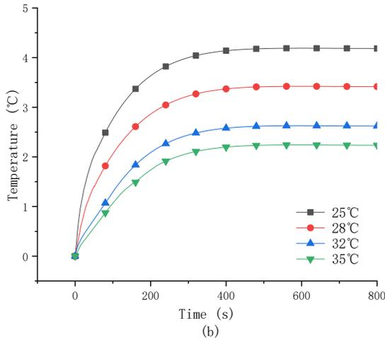
Fig. 3.  $\Delta T$  of the battery pack in case 1 (a) traditional dry-cooling (b) with wet pad
