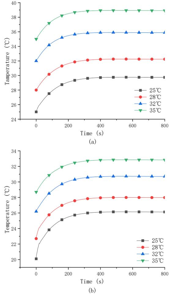
Fig. 2.  $T_{max}$  of the battery pack in case 1 (a) traditional dry-cooling (b) with wet pad
