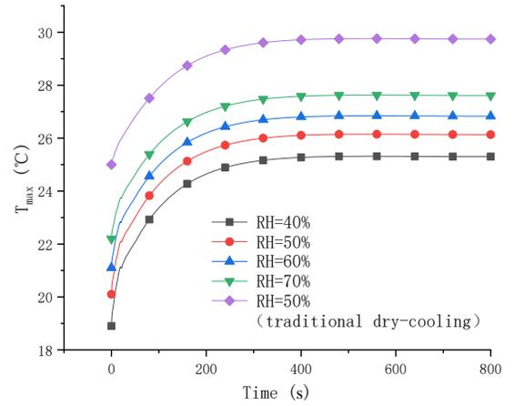
Fig. 4.  $T_{max}$  of the battery pack in case 2 (a) traditional dry-cooling (b) with wet pad
