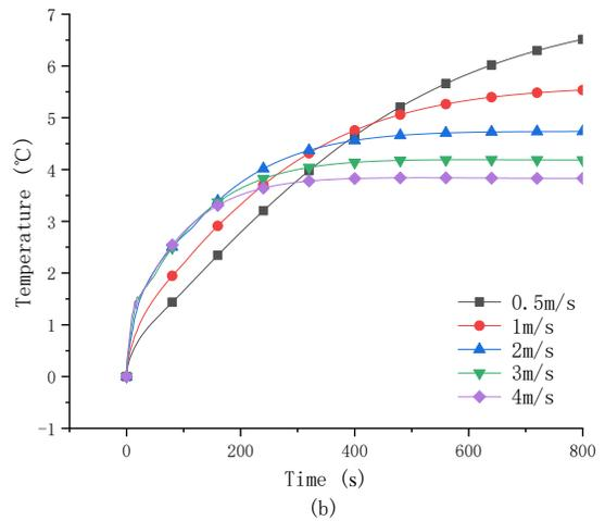
Fig. 7.  $\Delta T$  of the battery pack in case 3 (a) traditional dry-cooling (b) with wet pad
