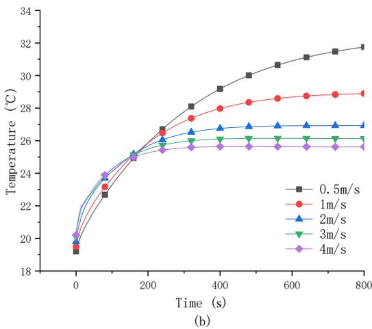
Fig. 6.  $T_{max}$  of the battery pack in case 3 (a) traditional dry-cooling (b) with wet pad
