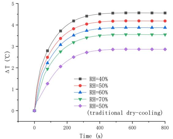
Fig. 5.  $\Delta T$  of the battery pack in case 2 (a) traditional dry-cooling (b) with wet pad
