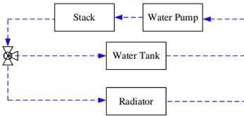
Fig. 2. The Cooling Circuit of fuel cell
