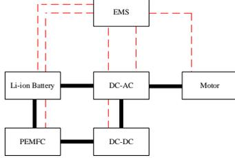
Fig. 1. The Structural schematic diagram of FCV
