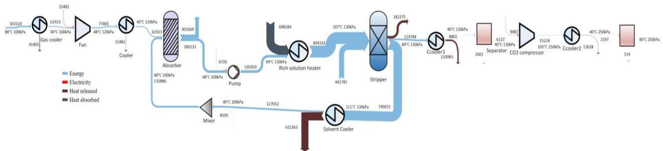
Fig. 3. Energy flow of CCS with compression
