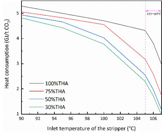
Fig. 2. Energy consumption varies with the inlet temperature
