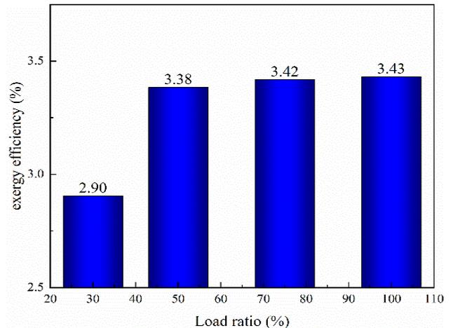
Fig. 5 Exergy efficiency of CPCC.
