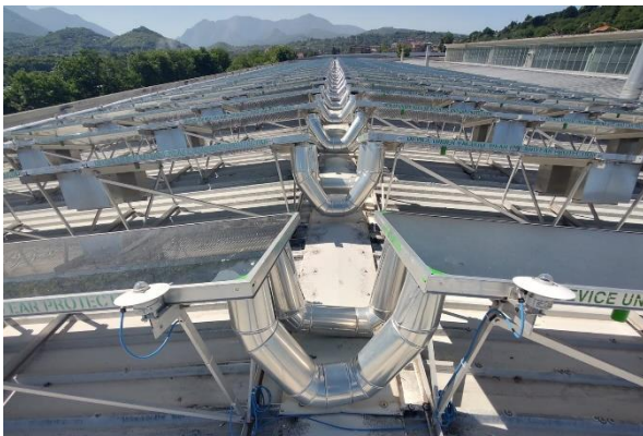
Figure 4 Arrangement of the two pyranometers for the second measurements campaign parallel to the panel surface
