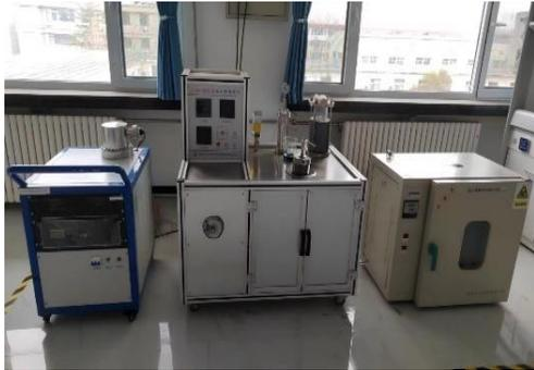
Fig. 1. ZTHJ-3A type rock pore casting instrument
