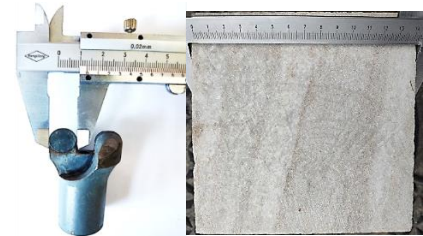
Fig. 3 Double-cutter PDC drilling bit and rock sample
