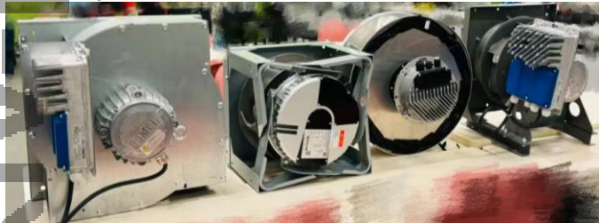
Fig. 2 Photos of the four EC fans tested in this study (Fan A, B, C, D from left)
