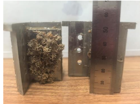
Fig.6 Bridging condition with Elastic Mesh Material
