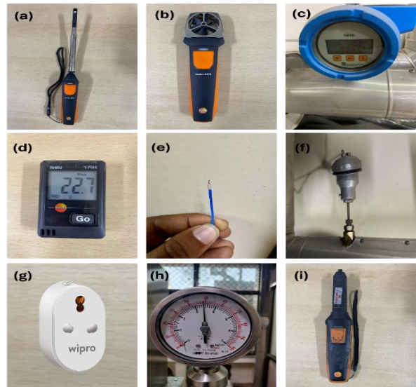
Fig. 4 Measuring instruments: (a) Hot wire anemometer, (b) Vane-type anemometer, (c) Turbine flowmeter, (d) Thermal hygrometer, (e) T-type thermocouple, (f) K-type thermocouple, (g) Wi-Fi smart plug, (h) Diaphragm gauge, (i) Air quality probe.
