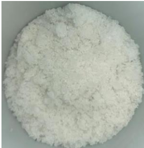
Fig. 2 40-60 mesh quartz sand mixed with ice particles
