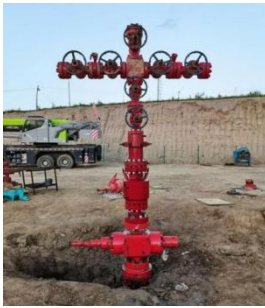
Fig.11. Test well completion wellhead
