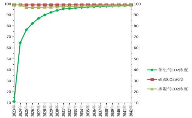
Fig.2. Purity of CO<sub>2</sub> after mixing CCUS-EOR associated gas with carbon source(mol%)
