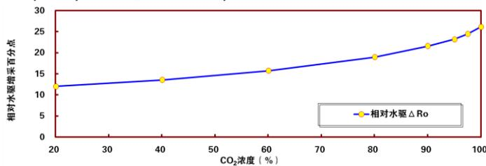
Fig.1. The relationship between the number of points increased in the numerical simulation recovery and the concentration of CO<sub>2</sub>
