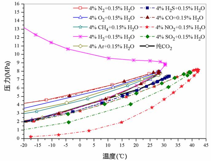
Fig.3. CO<sub>2</sub> fluid phase diagram containing impurities
