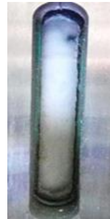
Figure 4. CO 2 mixed with APFR-4: 0.5%, APFR-R (cosolvent): 0.5%. Temperature: 90°C, Pressure: 20.69 MPa, Viscosity: ~20 mPa.s, State: homogeneous liquid phase
