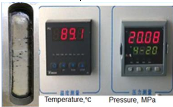
Figure 3(b) See-through cell showing a perfect proppant suspension (30 minutes without proppant settling).
