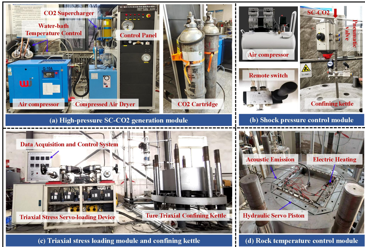
Fig. 2 Ture triaxial fracturing equipment for SC-CO 2 shock in high-temperature rocks. (a) High-pressure SC-CO 2 generation module; (b) Shock pressure control module; (c) Ture triaxial-loading module; (d) Rock temperature control in the confining kettle.
