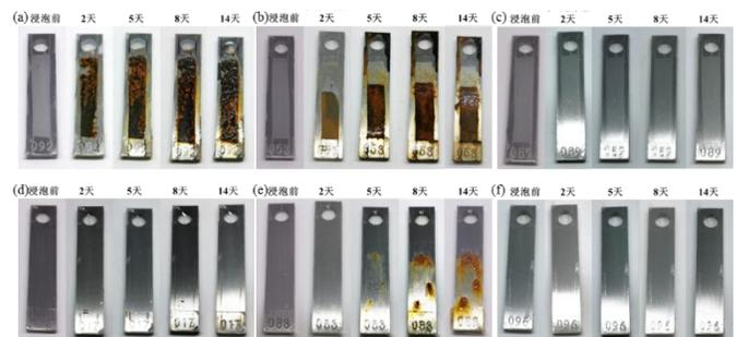
Fig. 1. Surface changes of coated and uncoated steel sheets after 14 days of reaction. (a) —uncoated, deionized water, (b) —uncoated, mineralized Water, (c) —uncoated, baked, (d) —coated, deionized water, (e) —coated, mineralized water, (f) —coated, baked
