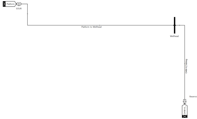
Figure 6: Integrated OLGA Model – from Platform to Bottom Hole
