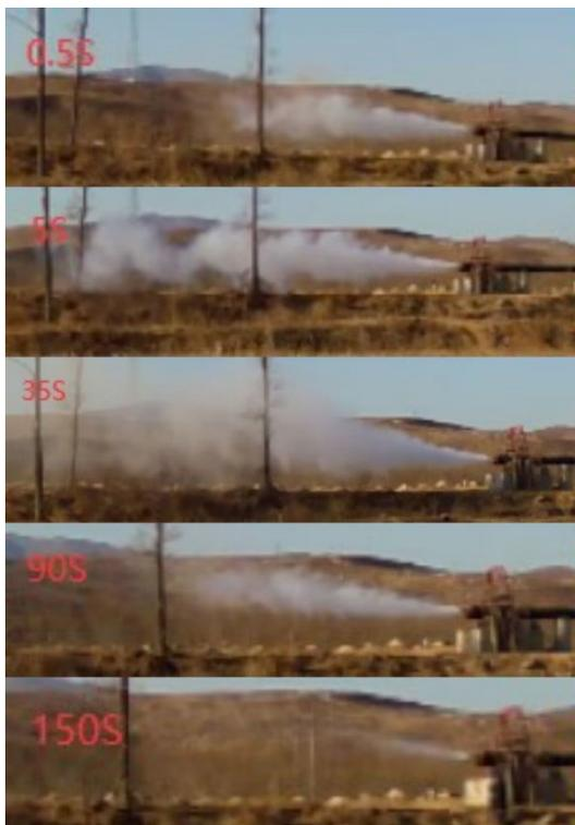
Fig.5. The jet morphology of 50mm aperture
