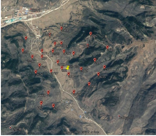
Fig. 4. Monitoring system in TS634 (red dots are the sensor positions, and yellow one is the injection well position)
