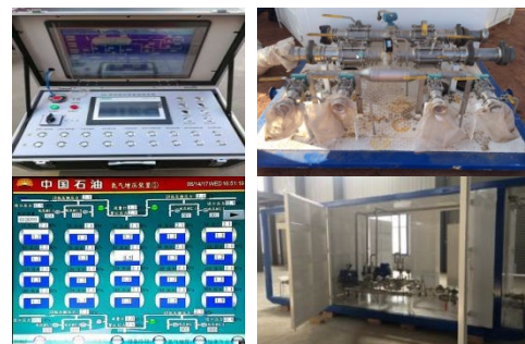
Fig. 3. N 2 pressurization device
