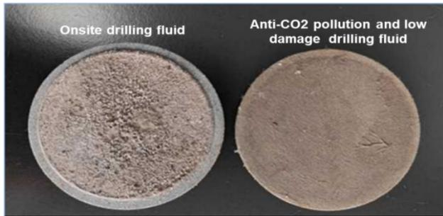
Fig. 8. (a) Pictures of plugging of 6700mD rock slab
