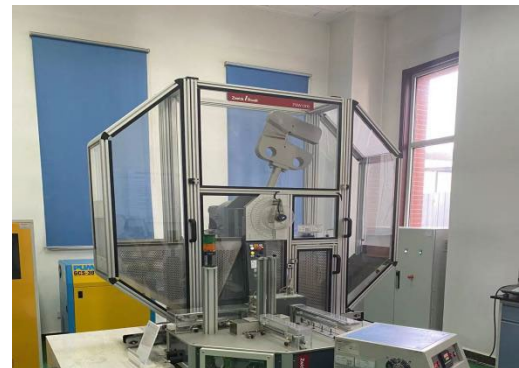
(a) Instrumented impact test
