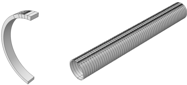
Fig. 7 Geometric model of supercritical CO 2 pipeline
