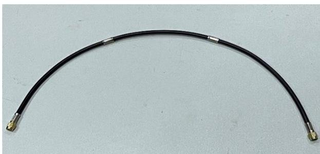
Fig. 2. CCFPI strain sensor made in laboratory
