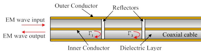
Fig. 1. Design of CCFPI strain sensor
