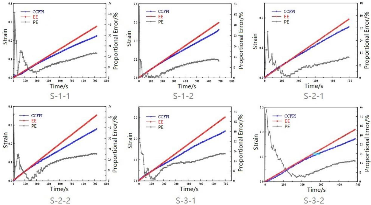
Fig. 4. CCFPI strain sensor vs. EE under different pretensions
