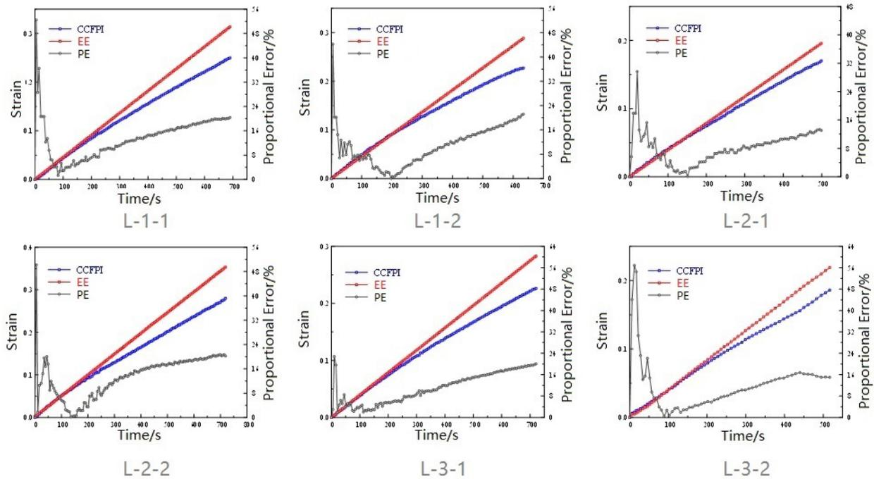
Fig. 5. CCFPI strain sensor vs. EE under different reflection point distances
