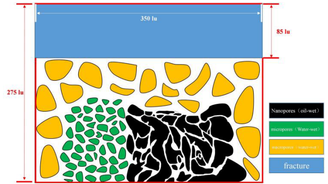
Fig. 1. Shale structure diagram ( including fracture, matrix ( organic matter, inorganic matter ) ).
