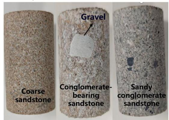
Fig. 1. The experimental cores
