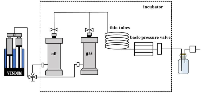
Fig. 3. Thin tube experimental setup
