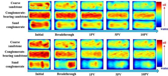
Fig. 4. Oil saturation changes during CO<sub>2</sub> displacement (upper panel) and CO<sub>2</sub>-WAG displacement (lower panel, 1:1 water-gas ratio) based on NMR imaging
