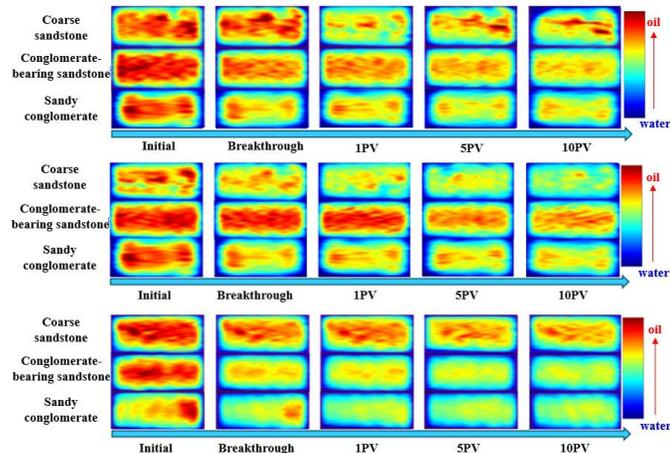
Fig. 8. Dynamic monitoring images of NMR under different water-air ratios (From top to bottom water-gas ratios of 1:2, 1:1 and 2:1, respectively)
