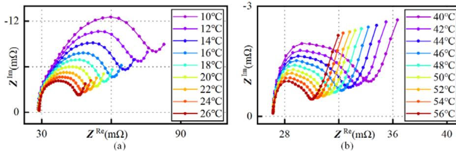
Fig.4 Reference EIS at different temperatures
