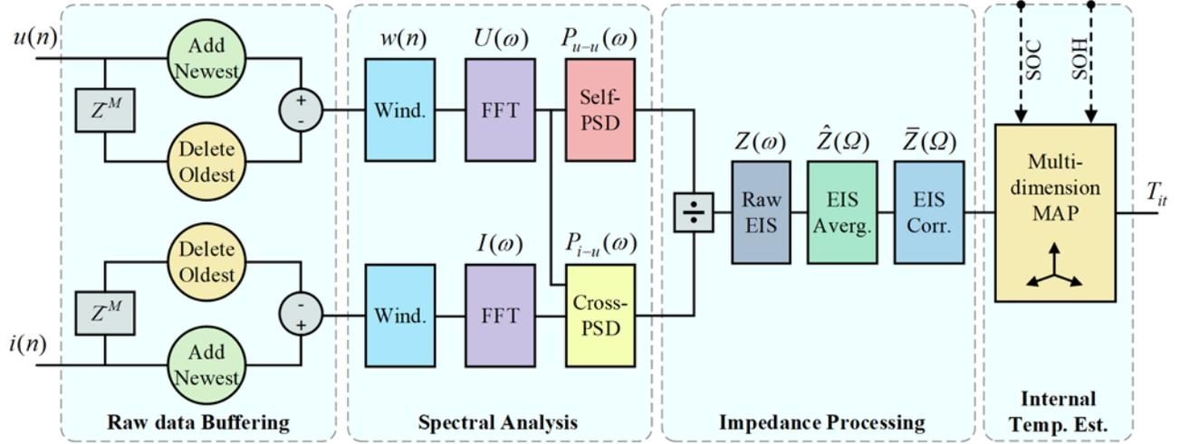
Fig.1 Procedures for acquiring passive EIS and internal temperature
