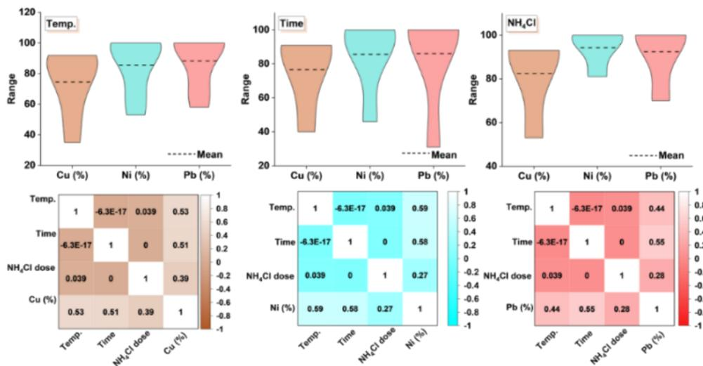
Figure 2. The data-distribution space of Cu, Ni and Pb recovery from the WPCBs with respect to the input variables: Temp., Time and  $\text{NH}_4\text{Cl}$  dose. The PCC based heat map constructed for Cu, Ni and Pb confirms the independent nature of the input variables.
