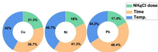
Figure 4. Significance of input variables towards Cu, Ni and Pb recovery from WPCBs using low-temperature roasting process.
