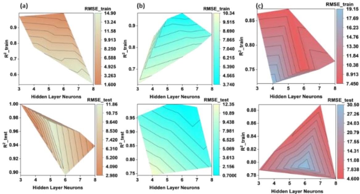
Figure 3. Development of ANN model for Cu, Ni and Pb recovery from WPCBs. The training and testing performance of the models having different hidden layer neurons are evaluated with respect to  $R^2$  and RMSE for a) Cu, b) Ni, and c) Pb.
