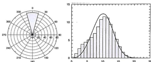
Fig. 3 Zafarana long term wind measurement and direction distribution [15]
