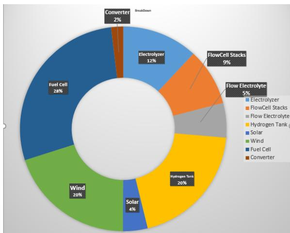
**Fig. 6 Cost breakdown at the best case**
