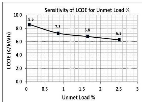
**Fig. 7 LCoE change with the unmet load percentage**
