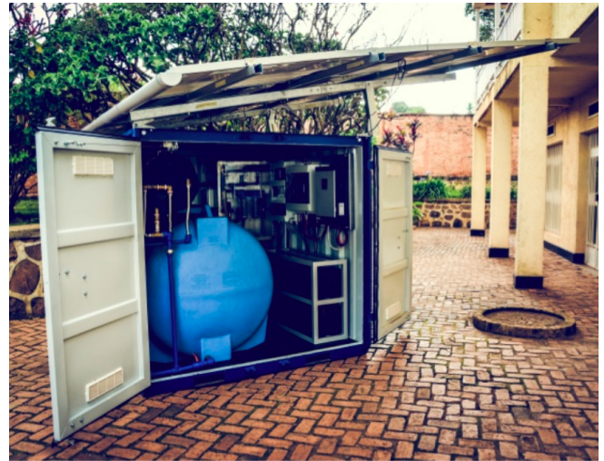
Fig. 3. Pilot design of the water purification system within the OGB system. It is composed of a 5-micron filter and an activated carbon/charcoal filter and a UV lamp. It also has a desalination option. The input sources can be rainwater, municipal water, groundwater or freshwater. The clean water can then be distributed in jerrycans, sachets, a smart-tap, or packaged water.
