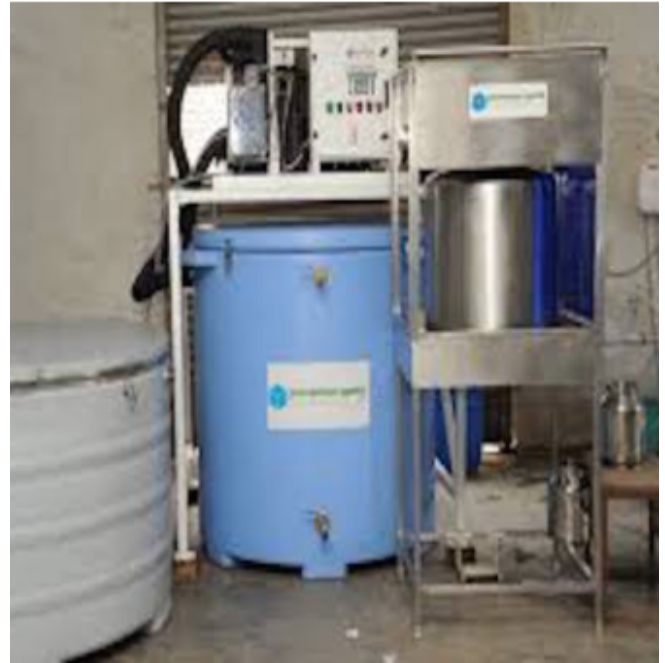
Fig. 4. The Promethean Rapid Milk Chiller is a modular system that cools milk from 35 degrees to 4 degrees Celsius with a capacity of 1,000 liters of milk per day. Such a system, paired with a Box (pending real-world compatibility testing) could significantly support Rwanda's dairy value chain as well as its aggressive childhood nutrition national strategy.
