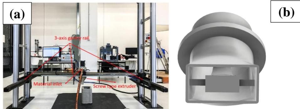
Fig. 1. Additive manufacturing of hollow-core element (a) 3D printer (b) nozzle for hollow-core printing
