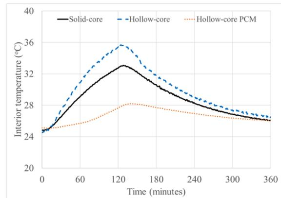
Fig. 5. Indoor temperature variation of simulated test rooms
