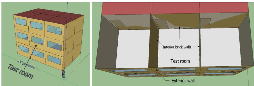
Fig. 4. Simulated building model (a) Thermal zones of the house (b) test room details
