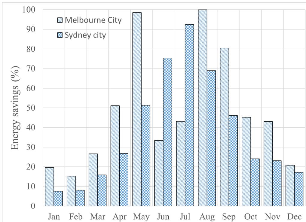
Fig. 7. Monthly cooling energy savings of hollow-core PCM panels incorporated buildings
