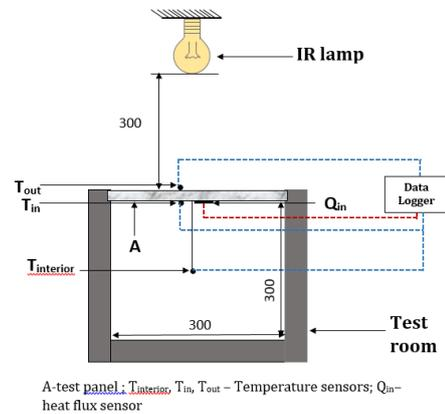
Fig. 3. Schematic diagram of simulated test room experiment
