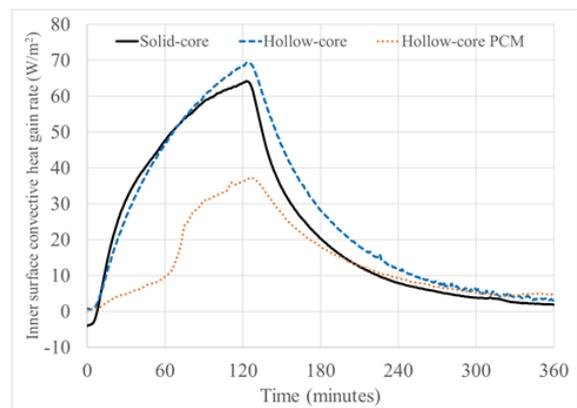
Fig. 6. Convective heat gain rates of panels
