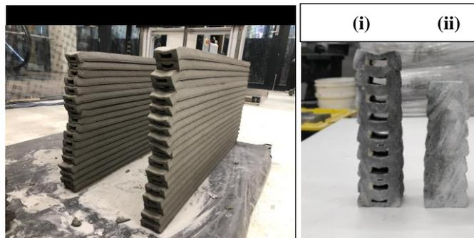
Fig. 2. Hollow-core printed specimens (i) hollow-core (ii) solid core
