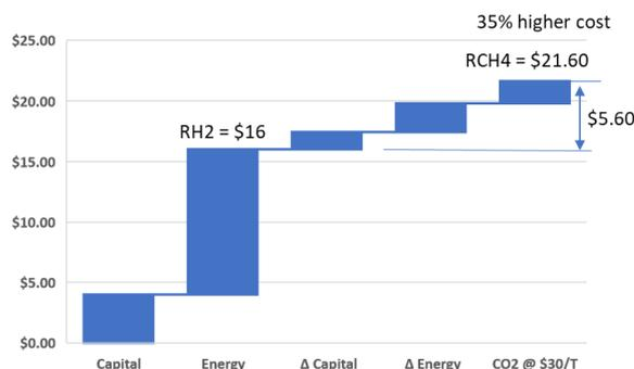
Fig. 3. Illustration of cost increments to produce methane from hydrogen
